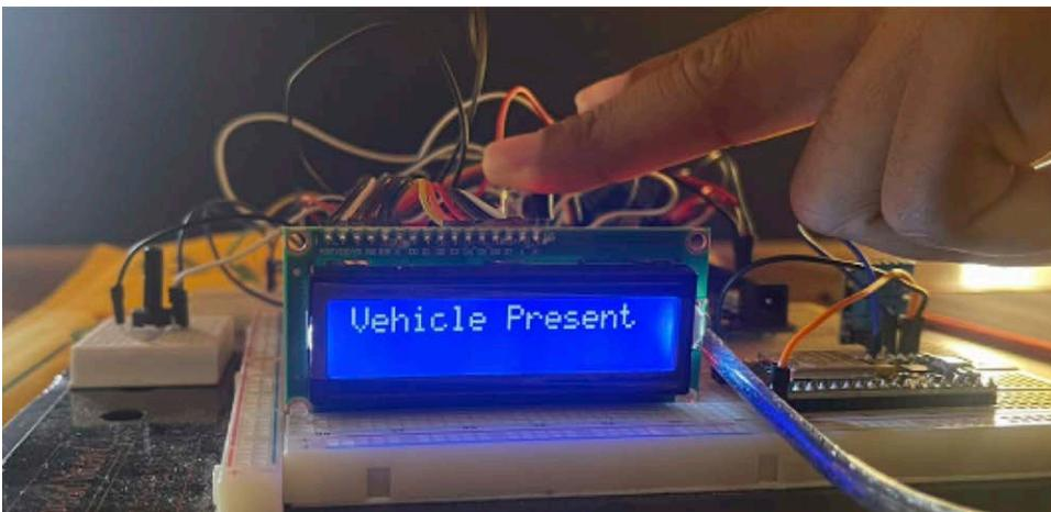
**Figure 2.** Display indicating the presence of a vehicle
