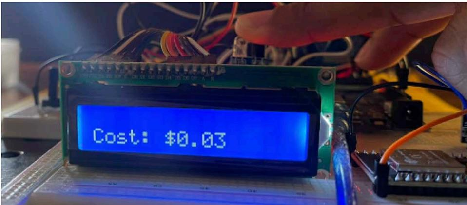
**Figure 7.** Display showing the cost at the end of charging
