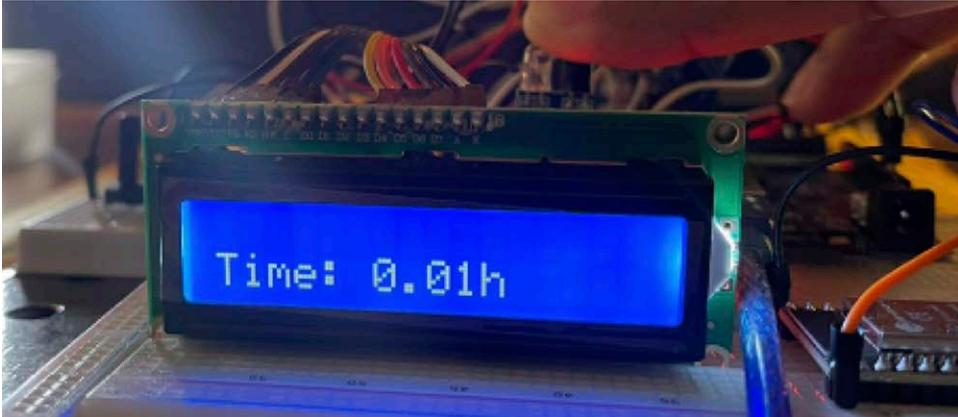
**Figure 6.** Display of the total charge time
