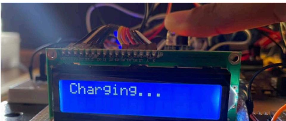
**Figure 5.** Display indicating charging in progress as the user has been authorized
