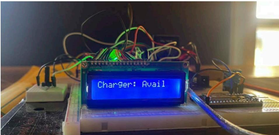
**Figure 1.** Display showing that a charger is available
